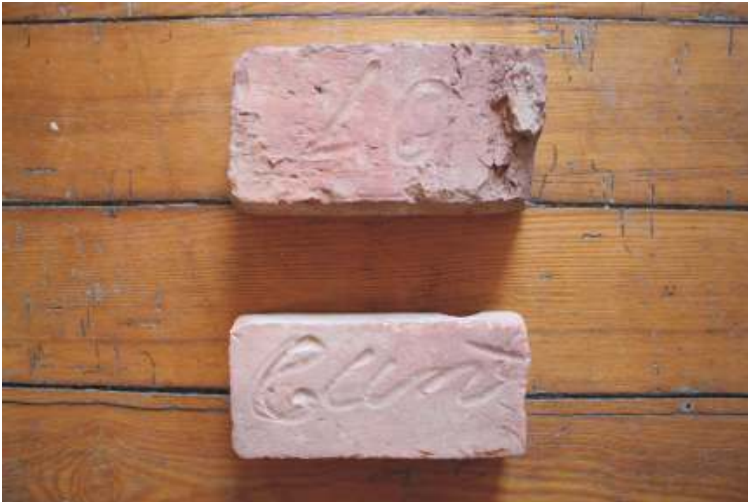
Figure 2. Large moppen bricks from the Peter McCutcheon House showing a) the inscription “40” and b) an incomplete inscription, possibly saying “Cutch.”
