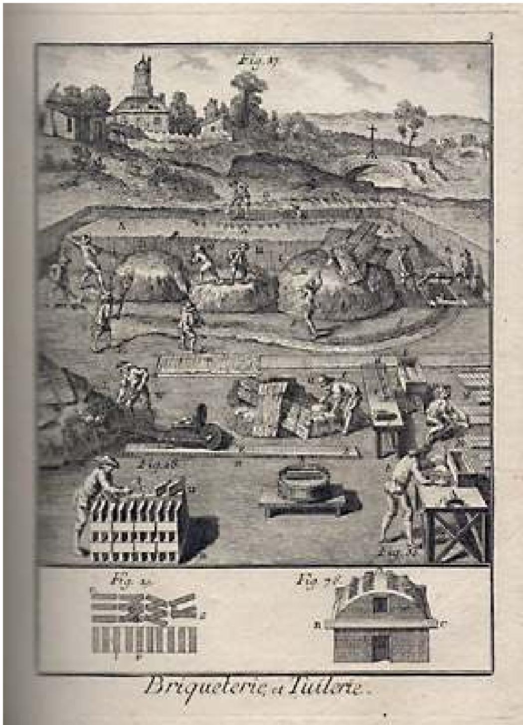
Figure 1. This engraving by Denis Diderot shows an 18 th century brickworks in operation, including the mining of the clay and molding of the bricks. Bricks manufactured for a small operation such the construction of a single house would undoubtedly be smaller in scale.
